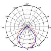
DM-TB2455WT-3545K Minimum Watt 30W Maximum Watt 40W PF 0.982 CRI 84 THD 11.8% Lumen 5000 Lm Efficacy (AC) 125 Lm/W 3500K Minimum CCT Maximum CCT 5000K Voltage Range 100-277V
