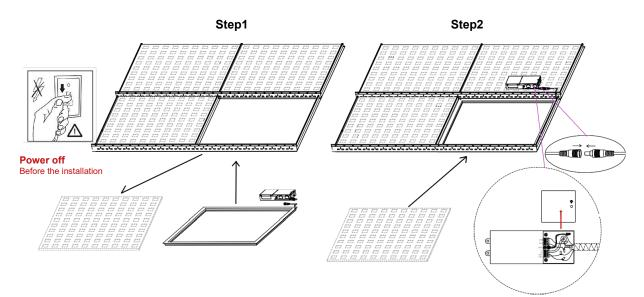
Step 1: Make sure of all the power is off before installing. Remove the one ceiling tile that you need to install light fixture on. Then place the light fixture on the T-bar carefully and make sure it is correctly in place and secure.
